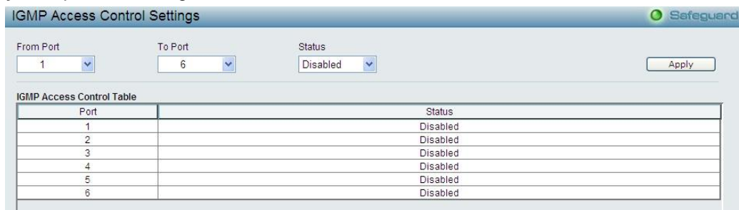
Figure 5.53 - Configuration > IGMP Snooping > IGMP Access Control Settings
