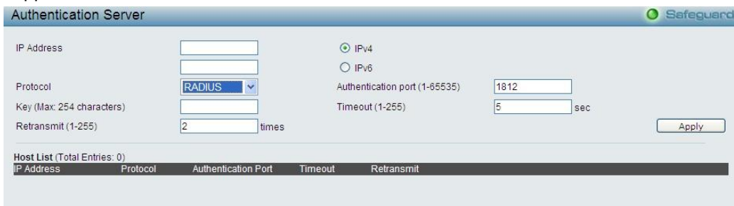
Figure 5.97 – Security > Access Authentication control > Authentication Server
