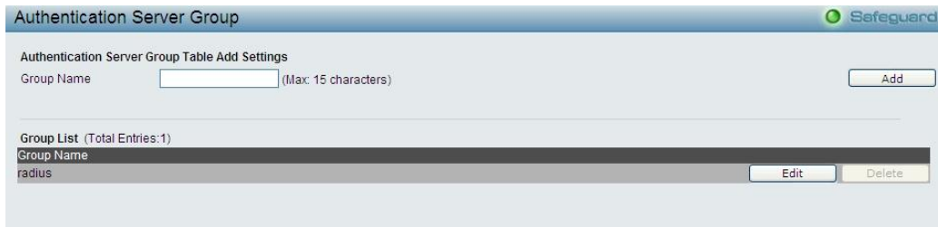
Figure 5.95 – Security > Access Authentication control > Authentication Server Group
