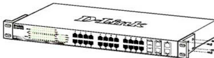
Figure 2.2 – Attach the mounting brackets to the Switch
