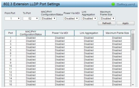
Figure 4.67 - L2 Functions > LLDP > 802.3 Extension TLV
