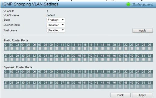
Figure 4.55 – L2 Functions > Multicast > IGMP Snooping VLAN Settings
