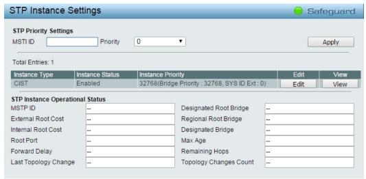
Figure 4.50 – L2 Functions > Spanning Tree > STP Instance Settings
