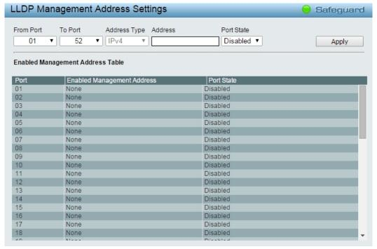
Figure 4.68 – L2 Functions > LLDP > LLDP Management Address Settings
