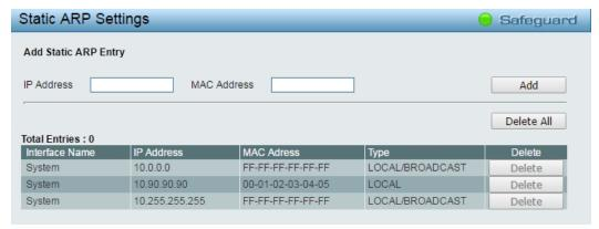
Figure 4.87 – L3 Functions > ARP > Static ARP Settings
