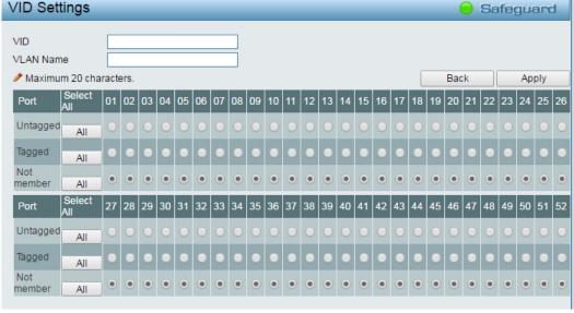
Figure 4.34 - Configuration > 802.1Q VLAN > Add VID
