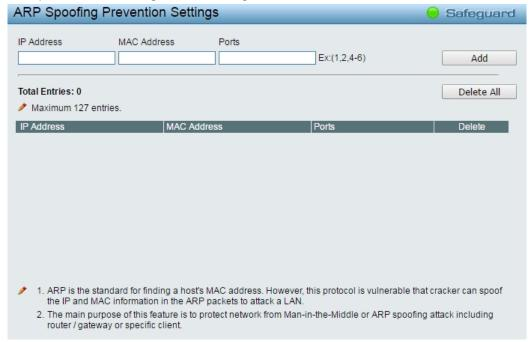
Figure 4.95 – Security > ARP Spoofing Prevention
