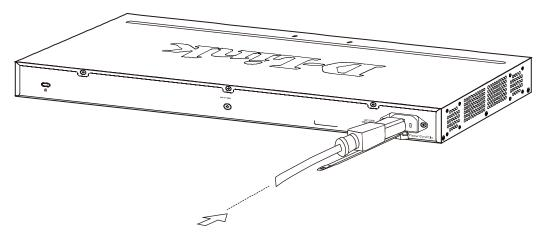
Figure 2.5 – Connect the power cord to the Switch
