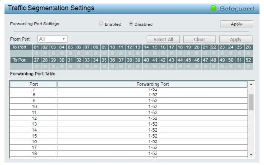
Figure 4.92 - Security > Traffic Segmentation
