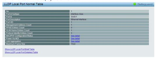
Figure 4.71 – L2 Functions > LLDP > LLDP Local Port Normal Table
