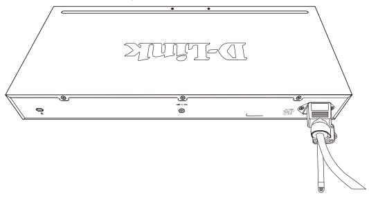
Figure 2.8 – Secure the power cord
