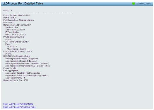
Figure 4.72 – L2 Functions > LLDP > LLDP Local Port Detailed Table
