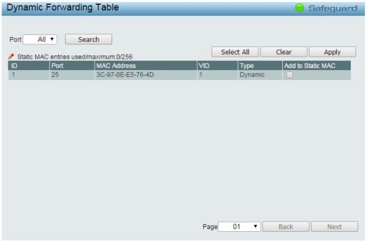
Figure 4.46 – L2 Functions > MAC Address Table > Dynamic Forwarding Table
