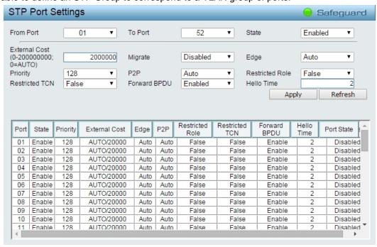
Figure 4.48 – L2 Functions > Spanning Tree > STP Port Settings
