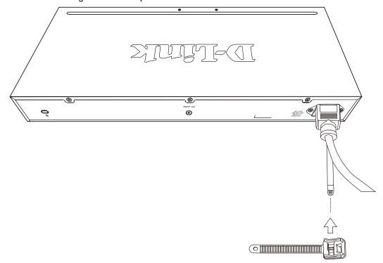
Figure 2.6 – Slide the Retainer through the Tie Wrap
