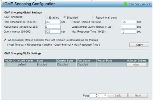
Figure 4.54 - L2 Functions > Multicast > IGMP Snooping
