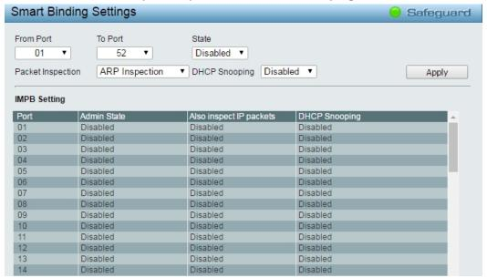
$Figure\ 4.104-Security > Smart\ Binding > Smart\ Binding\ Settings$
