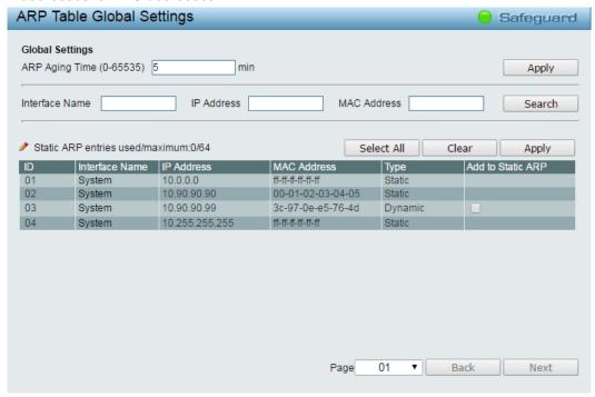
Figure 4.86 – L3 Functions > ARP > ARP Table Global Settings
