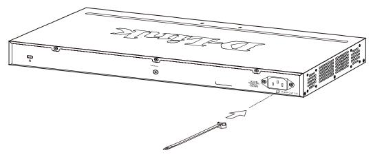
Figure 2.4 – Insert Tie Wrap to the Switch
