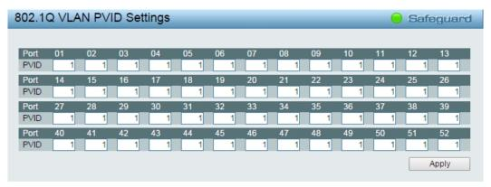
Figure 4.37 – Configuration > 802.1Q VLAN PVID
