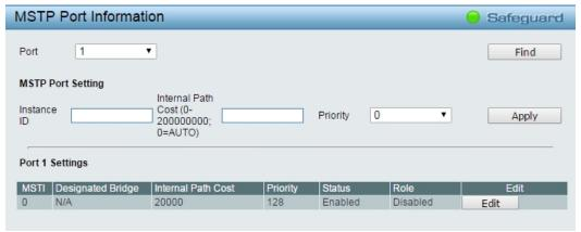
Figure 4.51 – L2 Functions > Spanning Tree > MST Port Information
