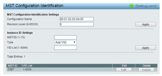
Figure 4.49 - L2 Functions > Spanning Tree > MST Configuration Identification
