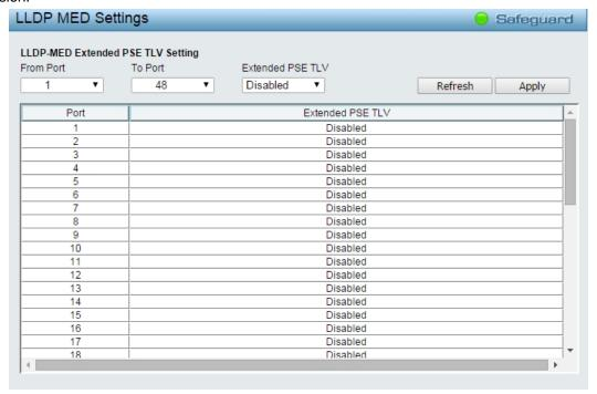
Figure 4.64 – L2 Functions > LLDP > LLDP-MED Settings
