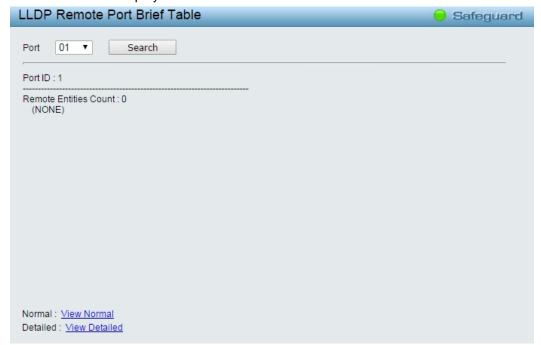
Figure 4.73 – L2 Functions > LLDP > LLDP Remote Port Table
