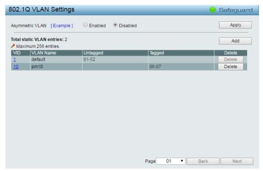
Figure 4.35 – Configuration > 802.1Q VLAN > Add VLAN
