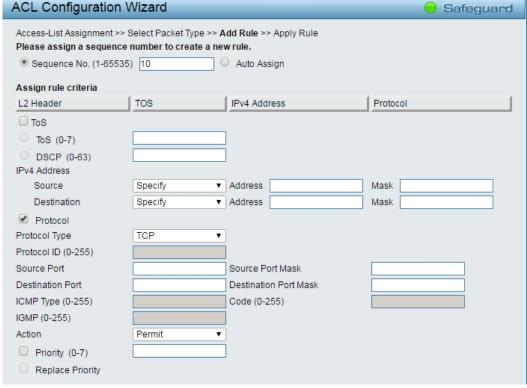
Figure 4.117 - Add Access Rule - IPv4 TCP
