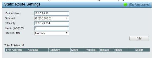
Figure 4.81 - L3 Functions > IPv4 Static Route - add
