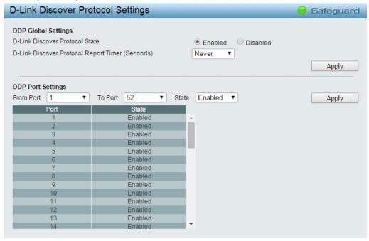
Figure 4.31 – System > D-Link Discover Protocol Settings
