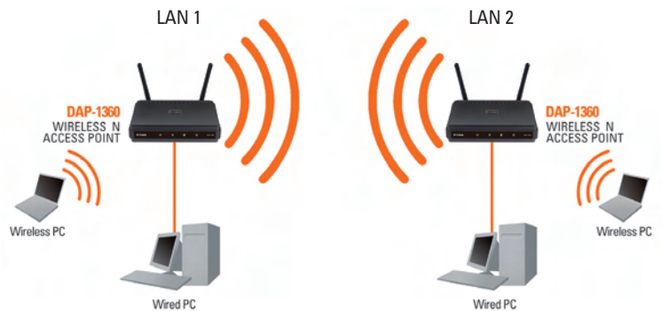
Connecting two separate LANs together through two DAP-1360 units (Wireless PCs can access the DAP-1360 units)
