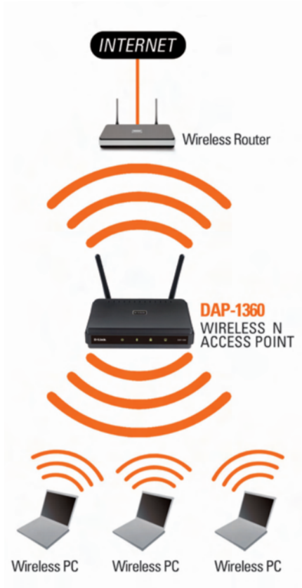
Extending the wireless coverage of a wireless router using the DAP-1360
