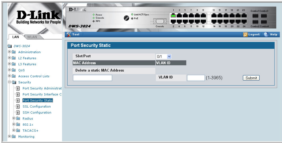
Figure 68. Port Security Statically Configured MAC Addresses
