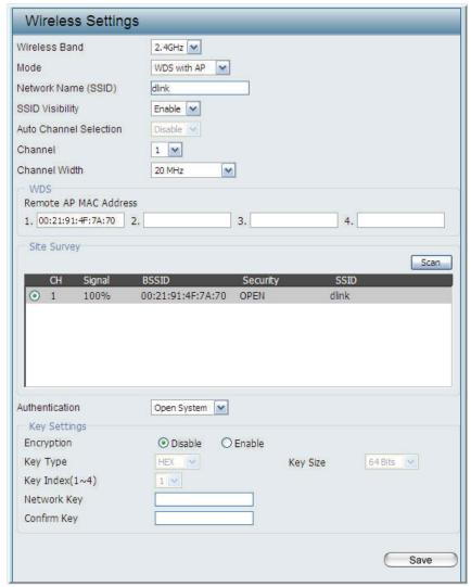
Remote AP MAC Address: Enter the MAC addresses of the APs on your network that will serve as bridges to wirelessly connect multiple networks.
