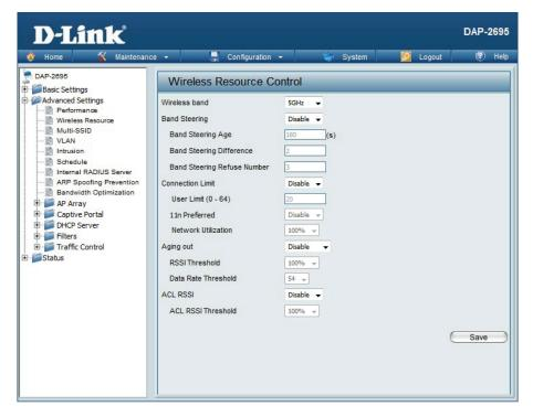
Band SteeringEnter the maximum 5GHz connection attempts allowed before the 5GHz preferred function will be disabled for the wire-Refuse Num:less station connection.
