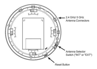
$\label{eq:Note: The DWL-6600AP has an internal antenna. If you would like to use external antennas, please slide the selector switch to the "EXT" position and attach the antennas.}$
