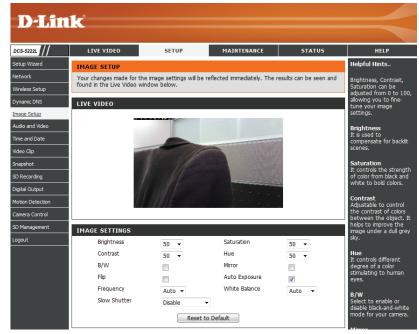
**Note:** *Mirror* and *Flip* can be used if you have mounted the DCS-5222L on the ceiling.
