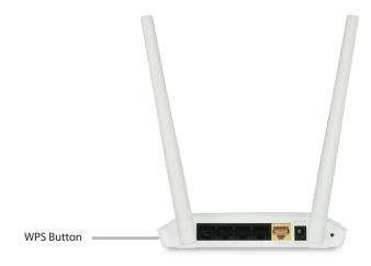
**Step 2** - Within 2 minutes, press the WPS button on your wireless client (or launch the software utility and start the WPS process).
